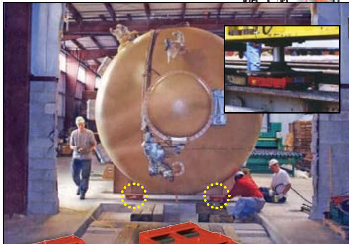
With 20 ton capacity, Hevi-Haul steel skate rollers can help move large equipment.
